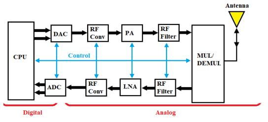
Figure 2. SDR block diagram with the receiver (lower part) and transmitter (upper part).
